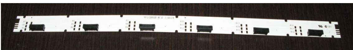
Figure 2: Flexible copper strip with straight sockets for Card LED
