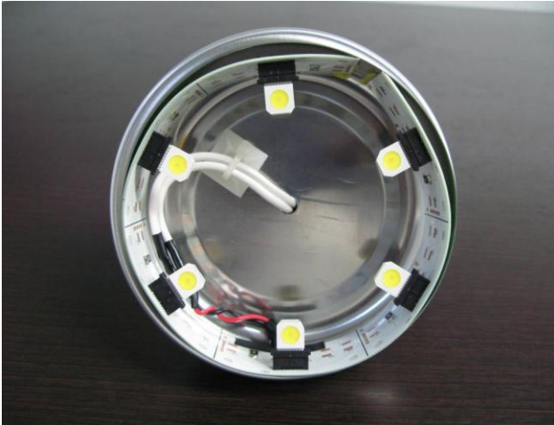
Figure 3: Circular downward array Card LED configuration in metal can.
